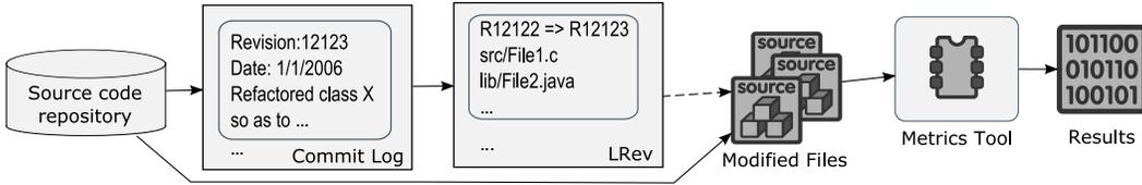
Fig. 9. The process used to evaluate the effect of refactorings
