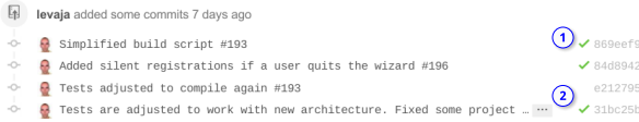
Figure 2: Integration of TRAVIS CI on GitHub, displaying build results in a pull request for multiple commits.
